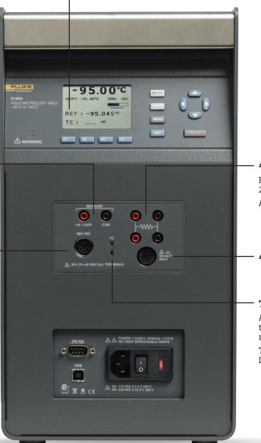
**4-wire PRT/RTD input** Reads a 4-wire, 3-wire, or 2-wire PRT/RTD Accuracy ±0.02 °C
