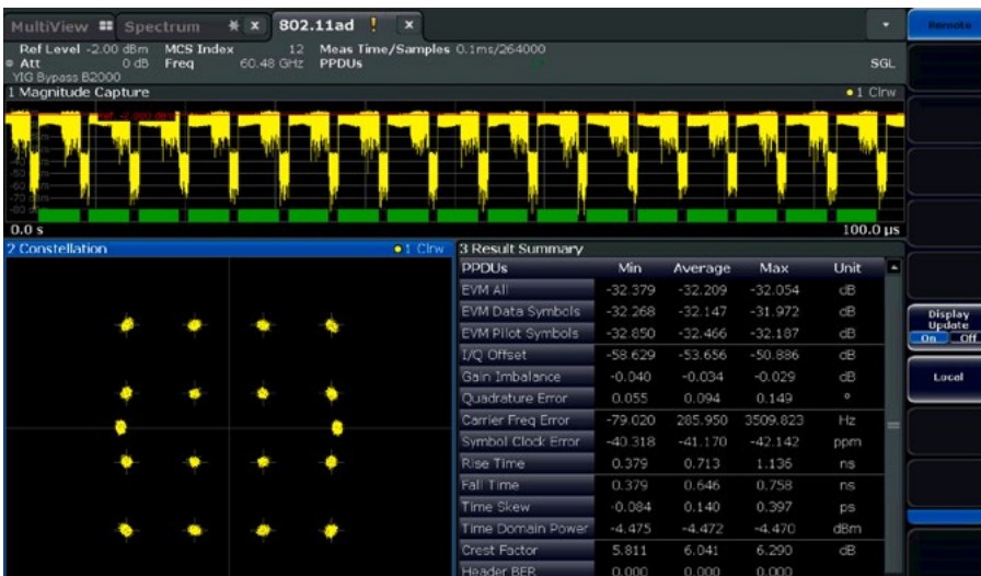
EVM of a WLAN IEEE 802.11ad signal (MCS12) at 60.48 GHz; measured with the R&S®FSW67 signal and spectrum analyzer.
