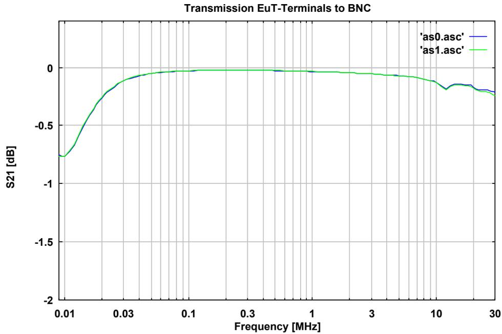
**Abb. 3 Transmission EuT – BNC**
